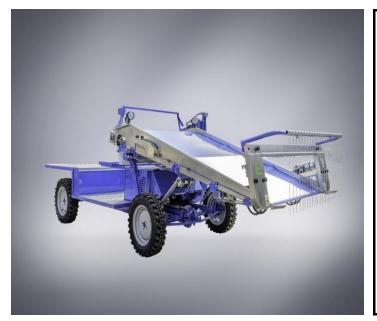
Ell-E is a totally electric zeroimpact harvester designed harvesting horticultural crops for cutting leaves. Ell-E is able to operate both under greenhouse and in open field and thanks to its compactness and driving, it is the ideal machine to make it work in environments where there are space problems. The machine has a working autonomy of more than 10 hours and it is possible to charge the battery pack with a common household socket, with a recharge cost of less than € 3.00
